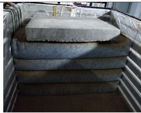
Figure 7. Wrap faced embankment
