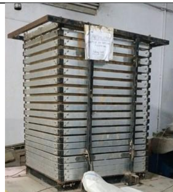
Figure 4. Laminar box mounted on shake table
