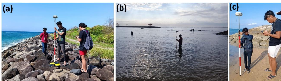
Figure 3. Coordinate measurements of GCPs and ICPs on ground (a), submerged ICPs (b), and water surface elevation (c)
