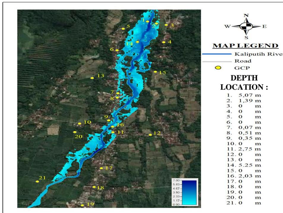
Figure 5. Flood inundation depth by HEC-RAS modeling
