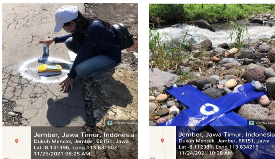
Figure 2. Marking and reading of GCP points
